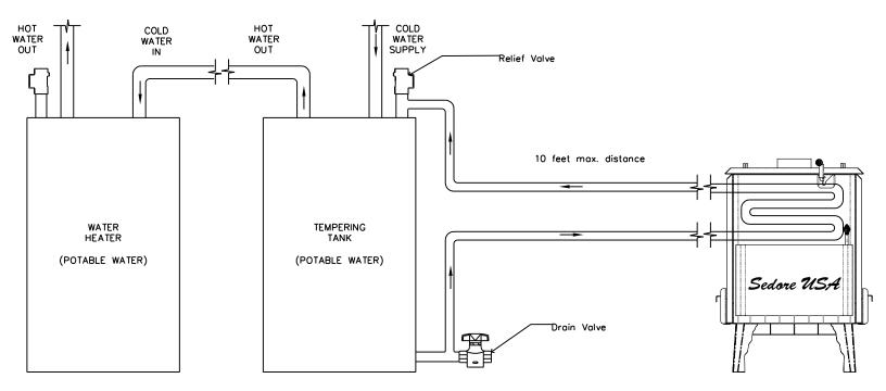
Install tempering tank as water heater method.
